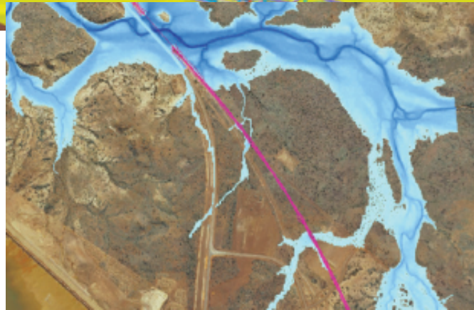
Image of 50yr flooding over aerial image (Duck Creek near top of image). Conveyor shown in pink lines.
